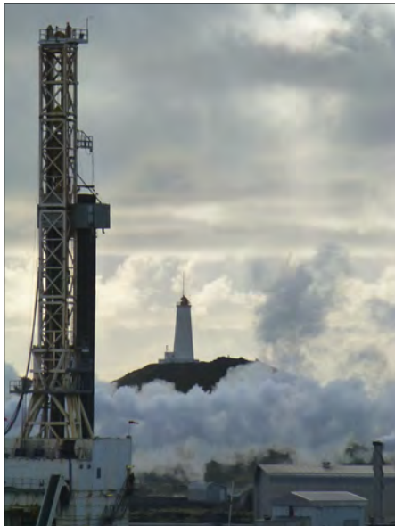
“The Power of Thor.” The rig used to drill well IDDP-2 at the Iceland Deep Drilling Project is named Thor. This supercritical drill hole shows the way to the future of geothermal power. At right is the lighthouse on the Reykjanes Peninsula, Iceland, showing the way to safe passage at sea. Photo by Robert Zierenberg, Davis, USA, July/Aug. 2018. GRC Photo Contest 2017
